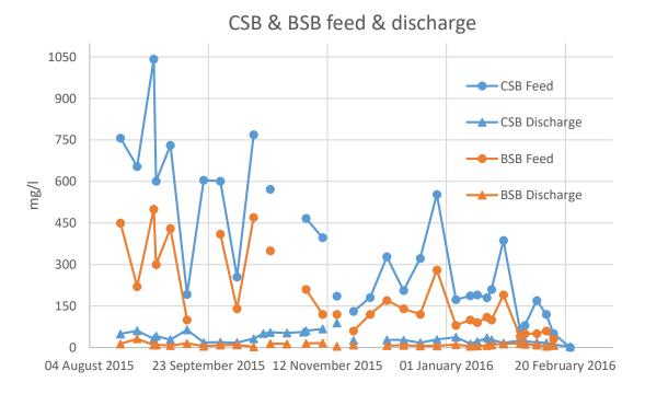
In the figure, the inlet and outlet values (COD and BOD) are presented for the pond treatment plant in the testing phase with the OLOID Type 400 with continuous reduction of aerator running times. Even at higher feed concentrations at the start of the test, the discharge values could be reliably maintained.
