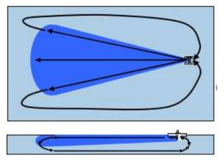
As a result of the impulse-like flow at an angle of about 30 ° from the OLOID in one direction, a flow similar to the heart is formed in the tank which encompasses and mixes the entire volume of the emulsion. This prevents the separation of the two media (water and lubricant) at standstill. These flow ratios are shown schematically in the left image.
